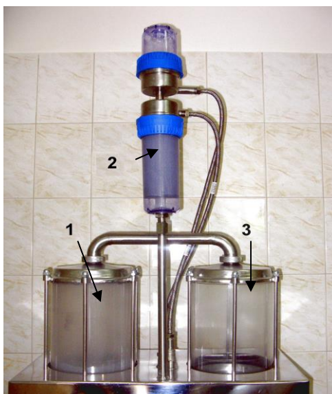
1 – a container to treat water with sorbent (sorption unit); 2 – a filtering element with a nanostructured membrane (membrane unit); 3 – a container for filtrate
